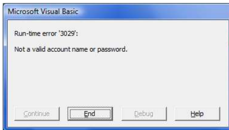
Figure 2-2: MF Decoder Error if You Start the Program Without Using the Shortcut
